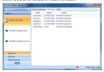
The **Diagnosis** application also lists all connected OMNIKEY smart card reader details (per the available contact and contactless interface).
