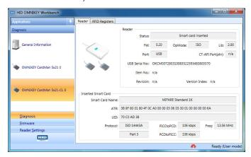
For a functional test, insert a working smart card into the reader. As a result, an ATR string and other card details will display.
